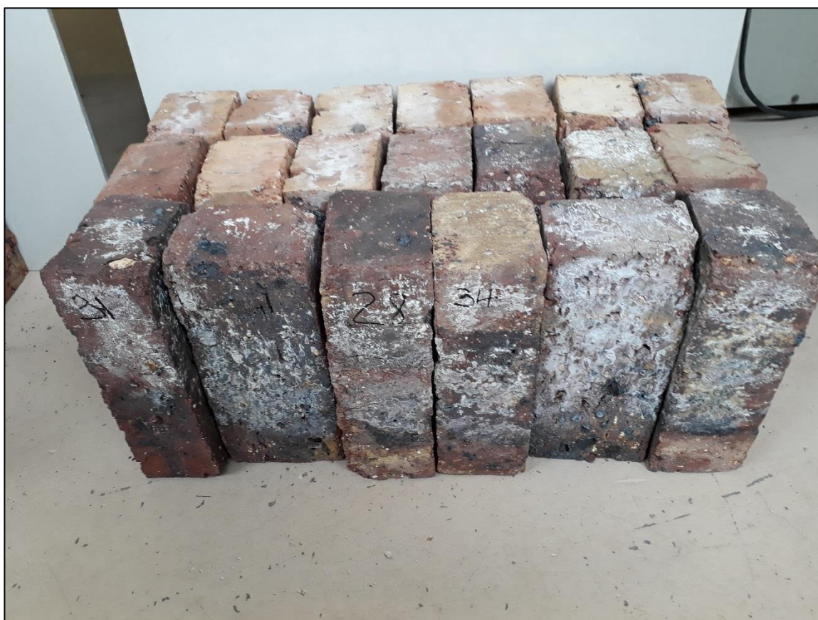
Figure 3.5.1: Samples after efflorescence testing
