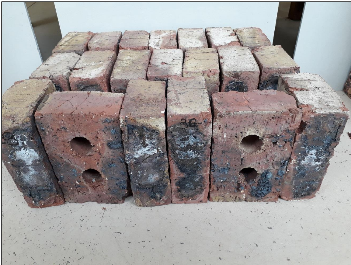
Figure 3.5.1: Samples after efflorescence testing
